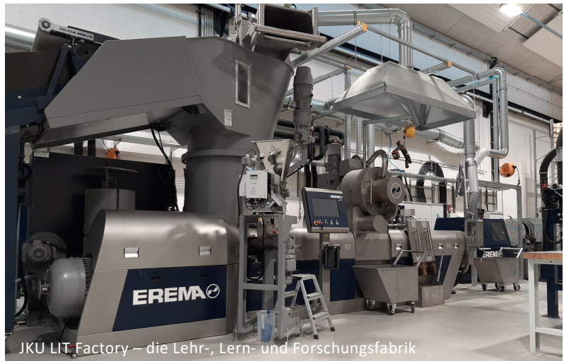
Recycling machine INTAREMA 1108 TVEplus (© CHASE/Chung)
