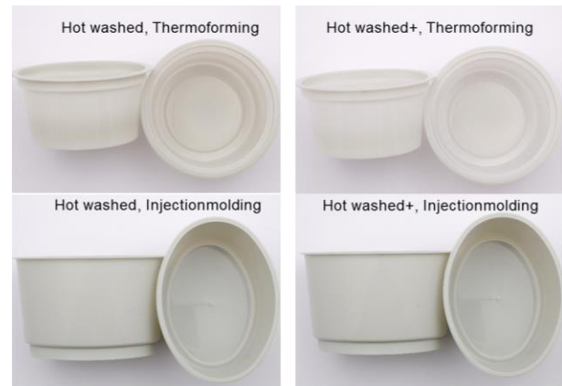
Figure 3: Images of the final cups, made of the recyclate after being subjected to different washing setups including hot washing (left) and hot washing+ (right). The cups were produced by thermoforming (top) and injection molding (bottom).
