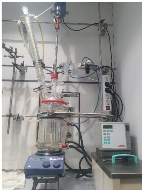
**Figure 3.** Experimental setup for washing experiments.
