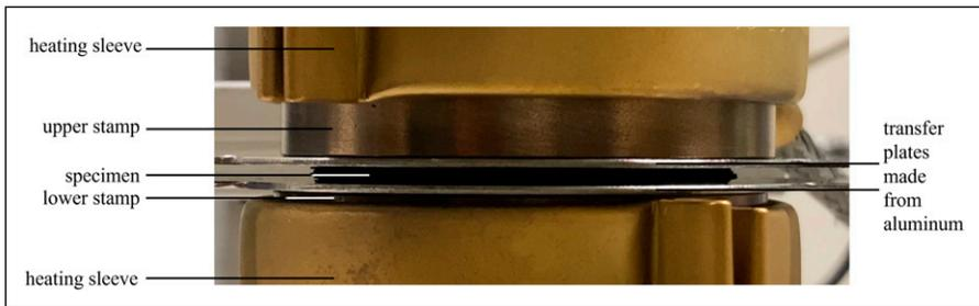
**Figure 7.** Frame of a video recorded during an experiment, showing the specimen, upper and lower stamps, the heating sleeves, and the transfer plates.
